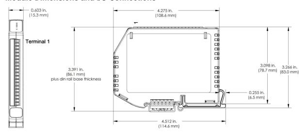
**Figure 1: Module Dimensions**
