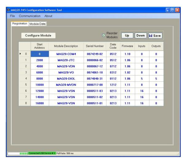
Figure 4: Module Registration using MAQ20-945 Configuration Software Tool
