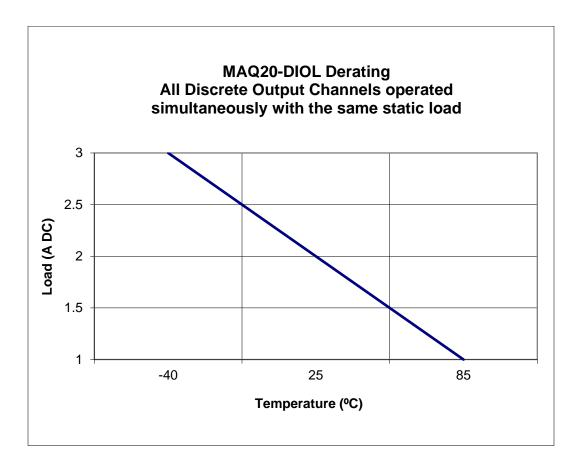
Figure 16: MAQ20-DIOL Derating for Static Loads
