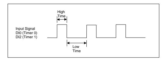
**Figure 10: Waveform Measurement Parameters**
