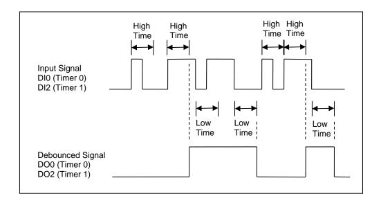
Figure 9: Pulse Counter with Debounce Operation
