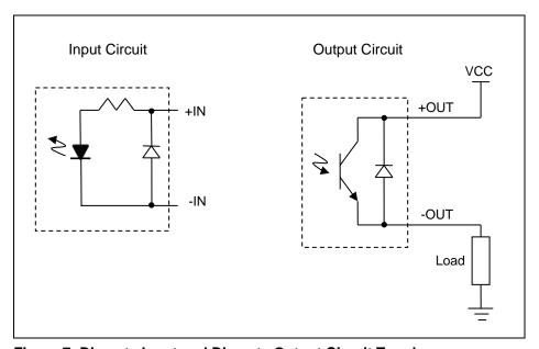
Figure 7: Discrete Input and Discrete Output Circuit Topology
