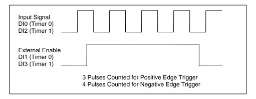
Figure 8: Pulse Counter Operation Using External Enable
