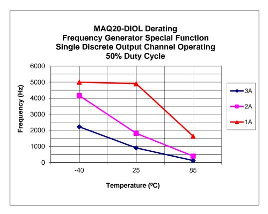
Figure 17: MAQ20-DIOL Derating for Single Channel Square Wave Output vs. Frequency
